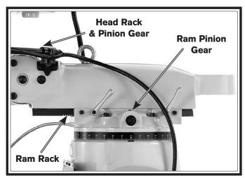
Figure 51. Locations of head and ram rack and pinion gears.
